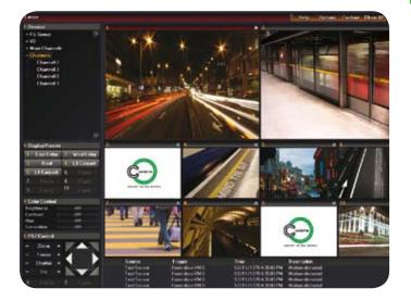
Cware Integra is an intelligent video management software that enables management and control of live and recorded video, integrating analog and digital video components. Cware Integra's all-in-one architecture is based on one standard PC serving as the recording server, system and client.
